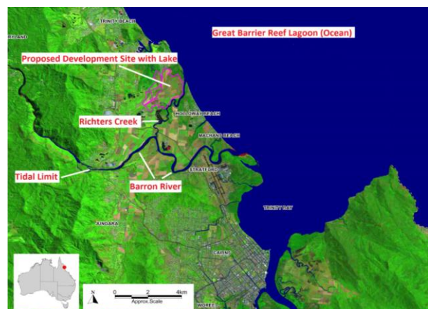
Figure 1 Location map. The development will consist of a 33 ha lake with ocean water cycled through with a 14 day residence time. Initially it was planned to discharge the lake water into Richters Creek near its entrance, presently the plan is to discharge directly into the ocean.
