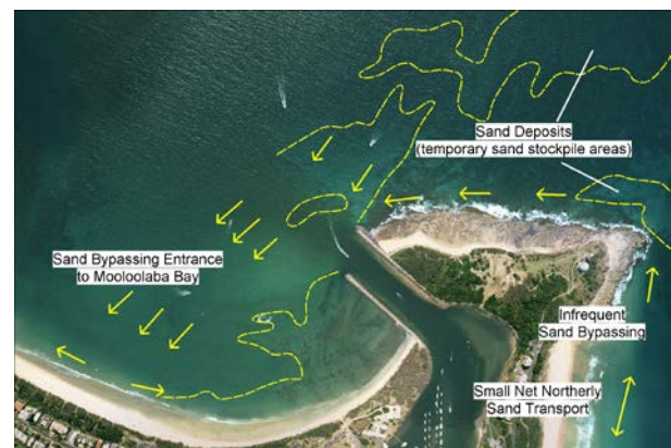
Figure 1 Conceptual model of sand bypassing at the Mooloolaba Harbour Entrance (modified from: [3])
