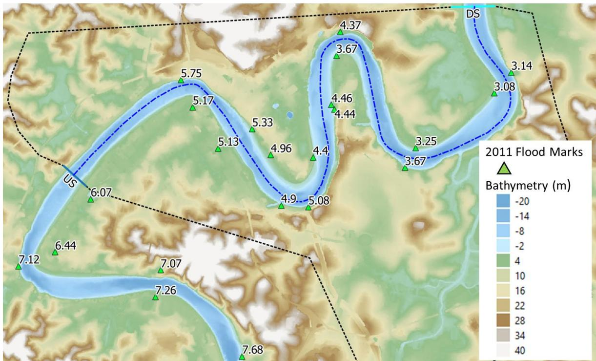
Figure 6. Brisbane River 5m grid bathymetry and the water marks during the 2011 flood
