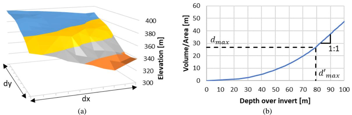
Figure 2. SGS implementation. (a) Example cell sub-grid elevation, (b) Cell storage function.
