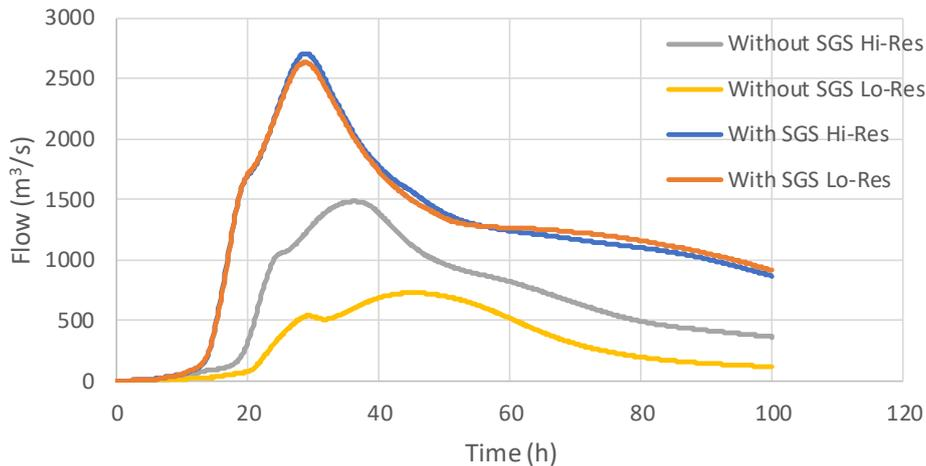
Figure 10. Direct rainfall whole of catchment cell size convergence with and without sub-grid-sampling
