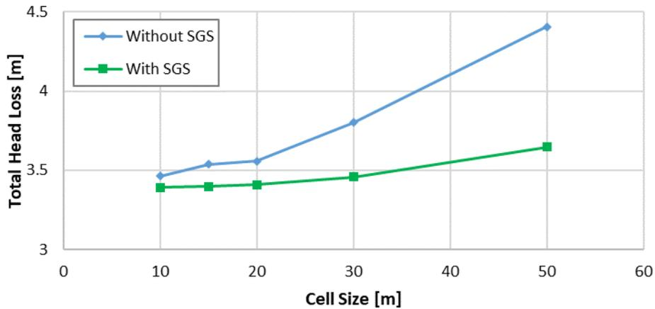
Figure 9. Brisbane River head loss with and without sub-grid-sampling
