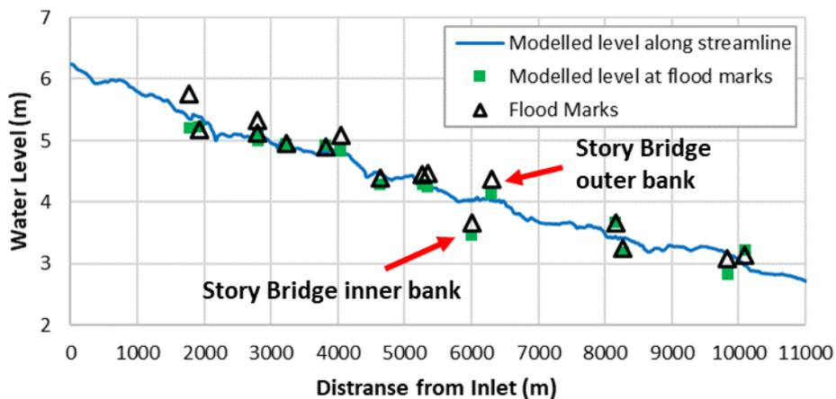
Figure 8. Simulated water surface along the streamline of Brisbane River compared with the flood mark
