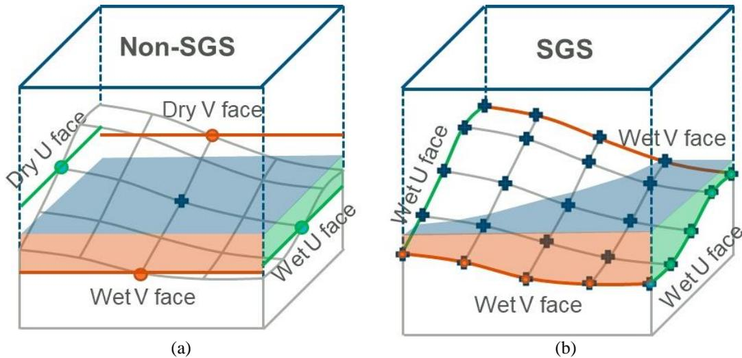
Figure 1. Regular 2D Mesh Terrain Sampling. (a) Traditional approach of a single elevation per cell centre and cell face. (b) Sub-Grid Sampling (SGS) at a higher resolution over the cell and across each cell face.
