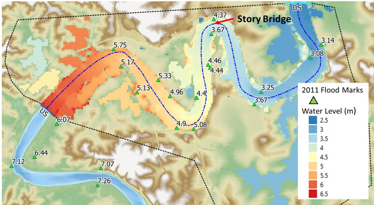
Figure 7. Simulated water surface level under 9000 m<sup>3</sup>/s flow vs 2011 flood
