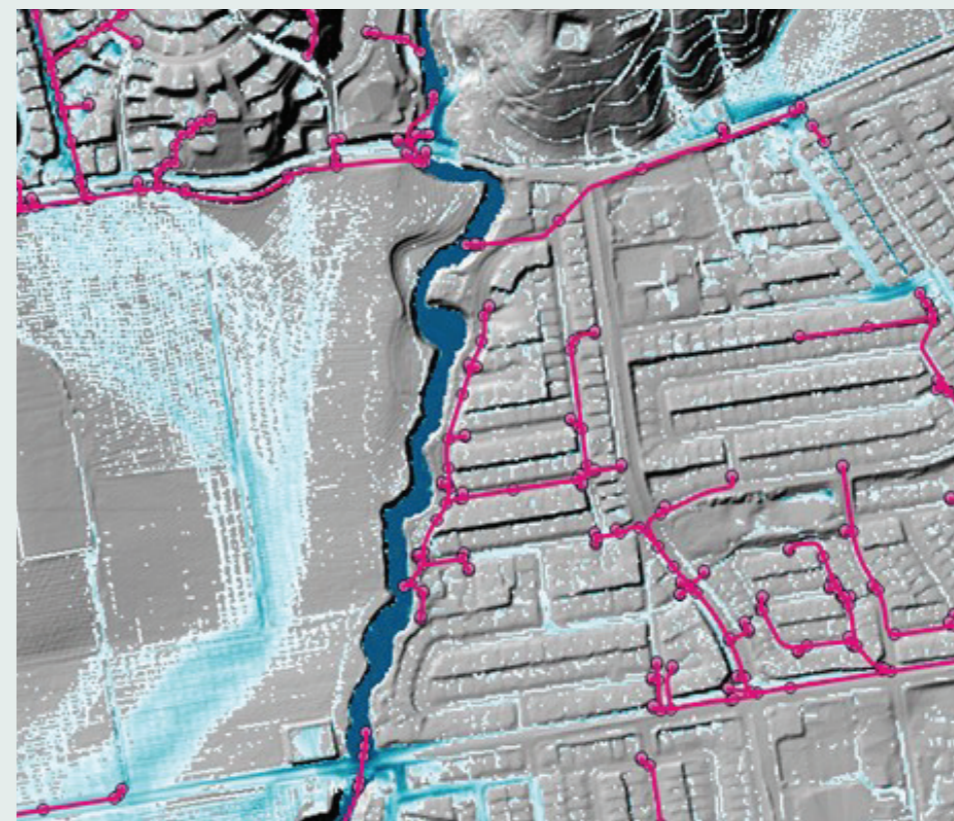
TUFLOW HPC Integrated 1D/2D Urban Drainage modelling
